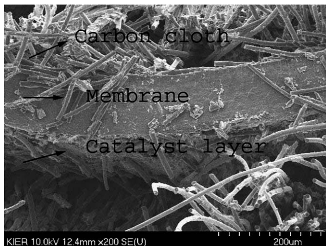
Fig. 4. SEM micrograph of cross-section of membrane electrode assembly.
